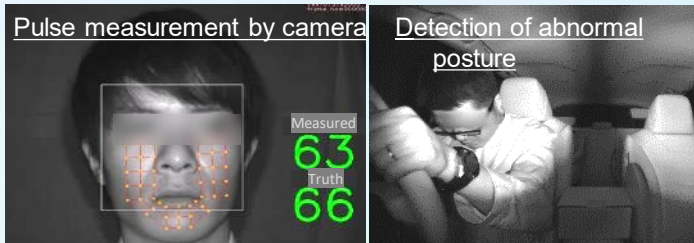
Vehicle automatically stops by detecting critical condition/ sudden sickness by non-contact pulse estimation, etc.
