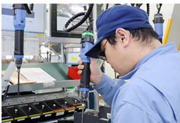
Lights on each screwdriver come on in the order in which they should be used.
