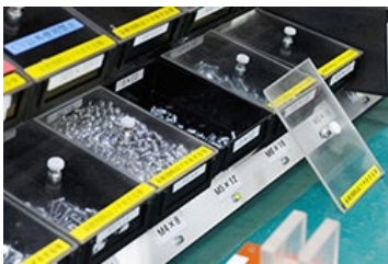
A light comes on to show which box components should be taken from.
