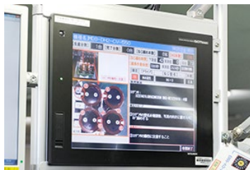
The display unit shows details of screw locations and sequence to prevent mistakes.
