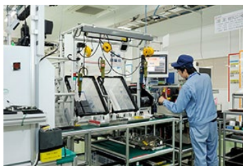
Cellular manufacturing facility producing PLCs and GOT HMIs.
