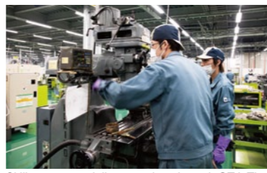
Skills are essentially passed through OJT. The photo shows a cemented carbide tool being machined by a worker during OJT.
