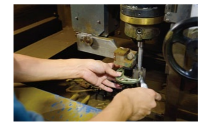
The wire-cut EDM robot system jointly developed with Mitsubishi Electric in 2013 to manufacture atypical electrodes. Playing an effective role in high-accuracy die manufacturing.
