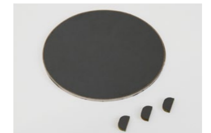
Diamond chips cut from a diamond wafer in a wire-cut electrical-discharge machine.
