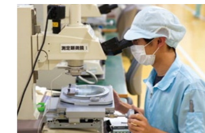
The die inspection process. Completed dies have a high machining accuracy of within \pm 1\mu\text{m} .
