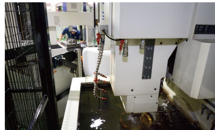
A 24-hour robot cell system with three Mitsubishi Electric DIAX EA12V EDMs, a robot conveyor made by Nichidai and a CMM.
