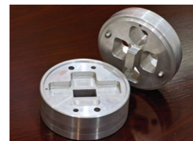
Die for aluminum extrusion. This die is subjected to over 5t of pressure to extrude aluminum sash frames.
