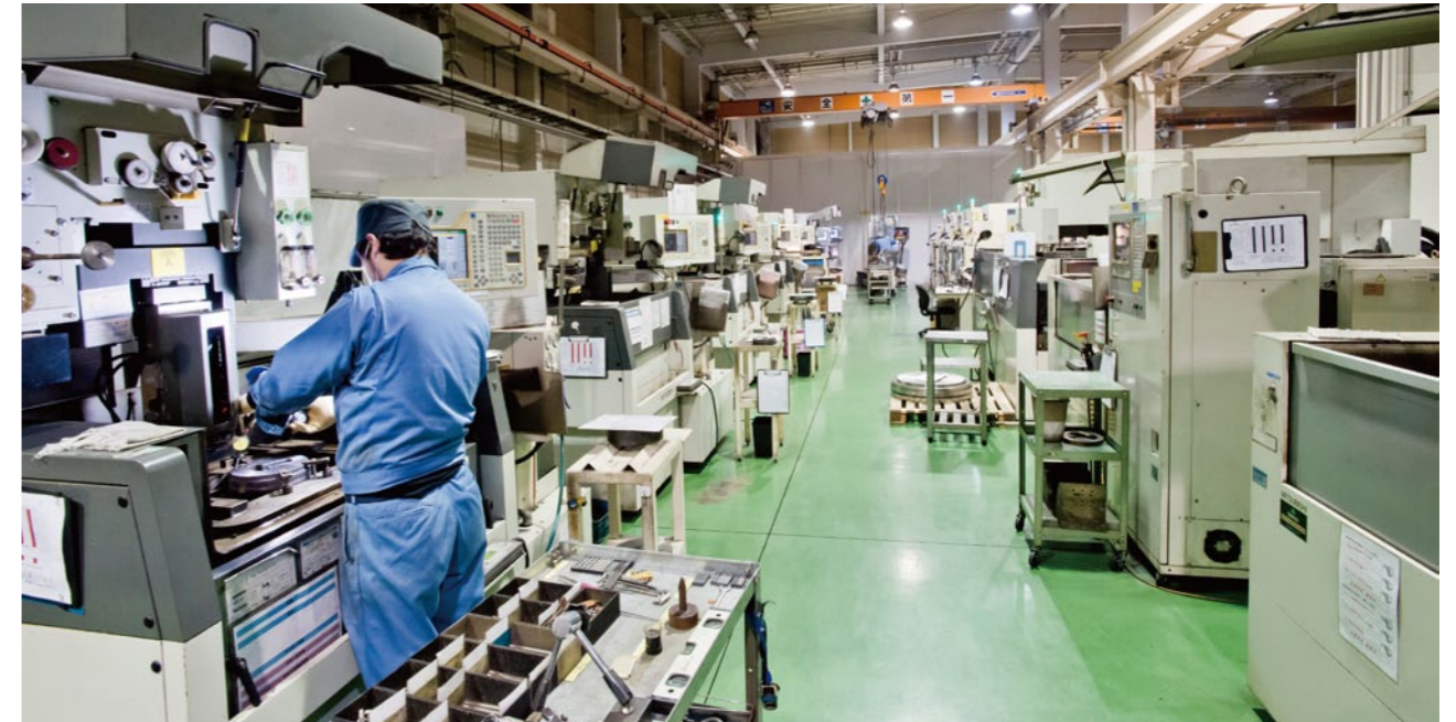
HSK's main plant for dies for aluminum extrusion, Atsugi Plant (Atsugi, Kanagawa Prefecture). A row of 40 EDMs.
