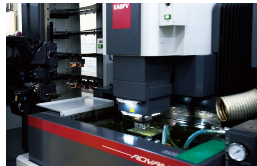
"EA8PV ADVANCE" is a die-sinking electrical-discharge machine (EDM) equipped with an automatic electrode changer—called an "ATC"—and workpiece changer. With Mitsubishi Electric's cooperation, the EDM is made to YUWA's specifications.
