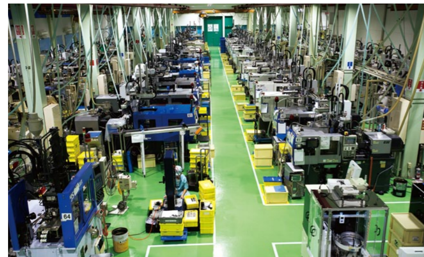
Plant 1 features a long line of 88 injection molding machines. In order to manufacture moldings for precision electronic components, the plant maintains an environment equivalent to a Class 100,000 clean room.
