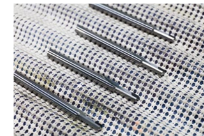
Diamond tools fresh off the manufacturing line. Made by soldering diamond chips onto a cemented carbide tool body.
