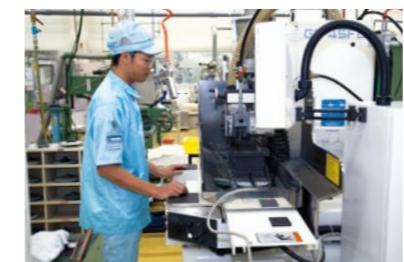
A grinder developed specifically for YUWA (both machine and grinding stone) in collaboration with the grinder manufacturer in order to achieve high accuracy.
