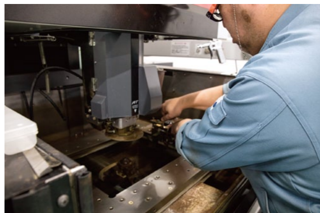
Manufacturing process for diamond cutting tools. Diamond blades for industrial use are processed in a wire-cut electrical-discharge machine (left) and accuracy is confirmed in a microscope. This process is repeated until the product is finished.
