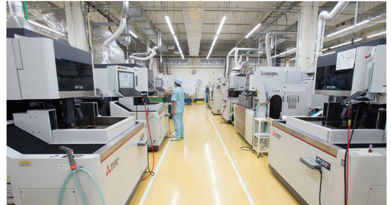
The wire-cut EDM line at the Die Technical Center is where YUWA manufactures its dies. The room temperature is maintained to within \pm 0.5^{\circ}\text{C} in order to secure high machining accuracy, and the machining water used is filtered rainwater that is almost entirely mineral-free.
