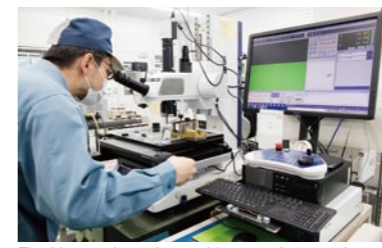
Final inspection prior to shipment. An experienced worker confirms processing accuracy by viewing a microscope image on an expanded display.
