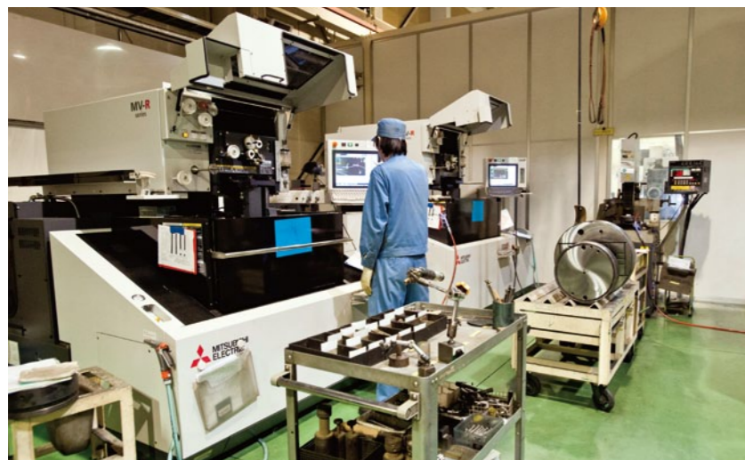
MV Series - The wire-cut EDM made by Mitsubishi Electric installed in the fall of 2015.
