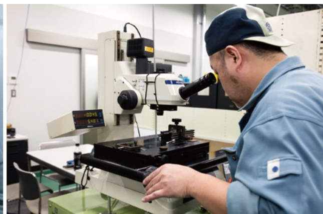
Manufacturing process for diamond cutting tools. Diamond blades for industrial use are processed in a wire-cut electrical-discharge machine (left) and accuracy is confirmed in a microscope. This process is repeated until the product is finished.
