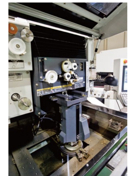
A wire-cut EDM processing dies for aluminum extrusion. HSK has top share of the market for this type of die.
