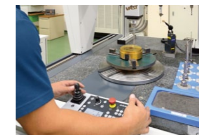
Final CMM measurement inspection of a cold-forging die manufactured in an EDM.
