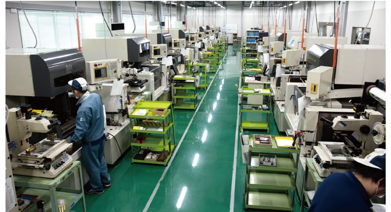
The diamond tool manufacturing line consisting of 20 wire-cut electrical-discharge machines, 19 of which are made by Mitsubishi Electric.
