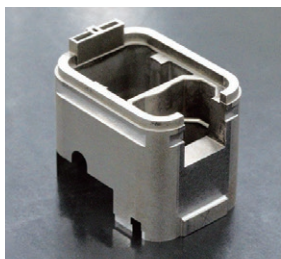
Sample of an injection mold die part. Wire machining and electrical discharge machining have been used for its production.
