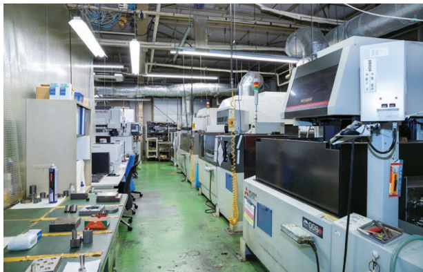
This production hall contains Mitsubishi Electric's EDMs: MV2400R, FA20, FA20P and FA20PS are on the right of the picture, with the ultrahigh precision MP2400 and EA12V on the far left. Kato Seisakusho is a longstanding Mitsubishi Electric partner and uses the company's processing machines as well as other products.
