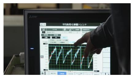
With a tool wear diagnosis system, data can be automatically collected to determine the optimal wear value, or tool life.
