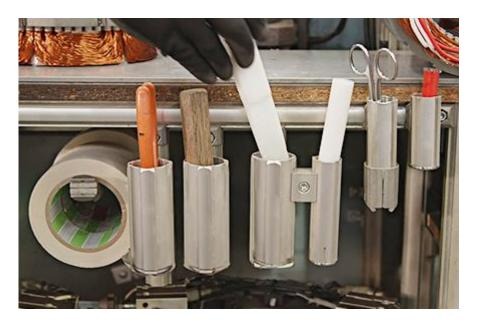
The work time was measured by attaching sensors to the tool holders
