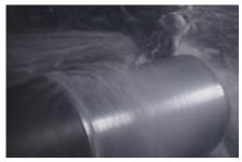
The final grinding process (right) was the bottleneck in the shaft production line. Closer integration with the preceding turning process helped to reduce the bottleneck (left).
