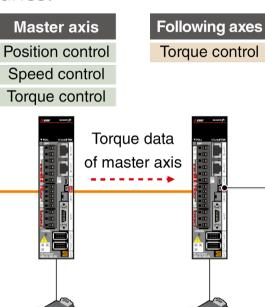
Drives the servo motor with the same torque as the master axis.
