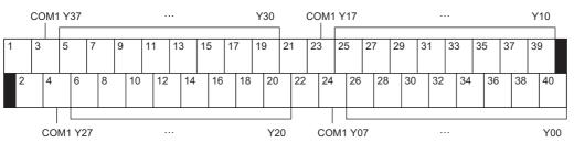
\*3 The FA-FXTH16YRA20S is equipped with an a-contact relay module. Replace with suitable triac or transistor modules (1 set of 4).
