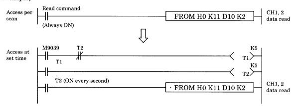
**Explanation:** By changing a program that reads data once a time at each scan into a program that reads the data only once per second, for example, the effect on the scan time and special function unit's processing time can be reduced.
