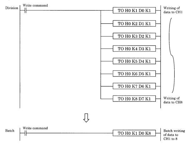
Explanation: With a program that writes data to eight channels, by executing batch read/write with one FROM/TO command as shown in the batch program, the effect on the scan time and special function unit's processing time can be reduced, compared to when executing eight TO commands as shown in the divided program.
