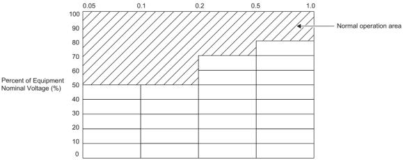
SEMI-F47 defines that equipment must be able to continue to operate without interruption during voltage sags shown in the above shaded area (voltage sag immunity).
