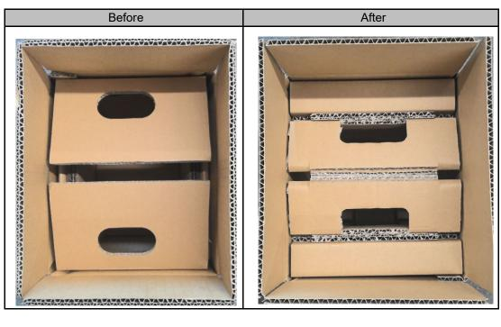
Appearance of the hand hole on each side of the packaging box for the FR-HEL-H5.5K to H11K
