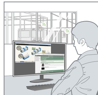
Work reports and equipment pictures saved in multiple (up to 50) GOTs can be displayed collectively on a PC for data management
