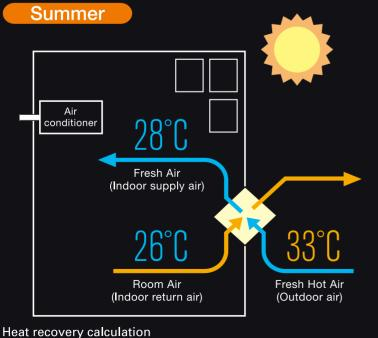
temperature (°C) × Temp recovery Indoor supply-air = Outdoor Outdoor temperature (°C) temperature (°C) temperature (°C) Calculation example:  $28^{\circ}\text{C} = 33^{\circ}\text{C} - (33^{\circ}\text{C} - 26^{\circ}\text{C}) \times 71.5\%$
