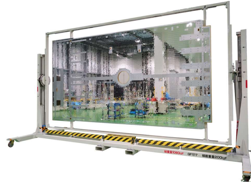
Heat Pipe Panel with OSR Installed
