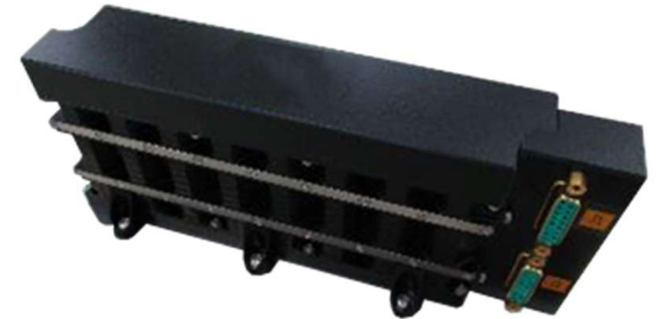
2P-8S 18650 Cell Battery with Overcharge Protection Circuit for RAISE-2 Satellite
