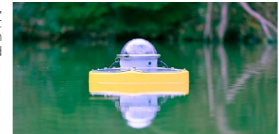
MINAMONITOR (Buoy type water surface sensor)
