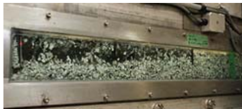
Water process for separating a mixture of shredded plastic pieces. Some types sink and others float to the water's surface. This water is recycled perpetually in the process.
