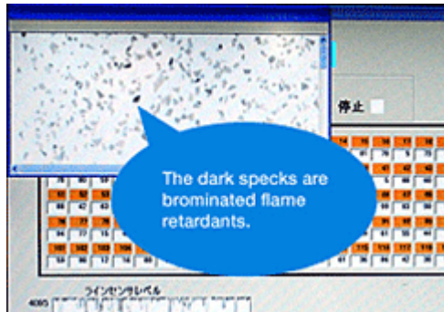
The equipment uses X-rays to identify flame-retardant plastic with an analysis speed of 120 seconds and removes it with 124 air guns. The technology received the Environment Minister's Award for Excellence from Japan's Ministry of the Environment.
