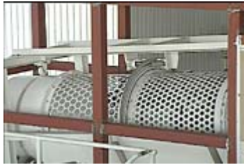
Sorting equipment High-capacity sorting of machine-crushed chips into three sizes
