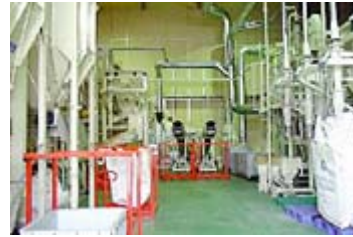
Proprietary fine-crushing equipment Plastic particles crushed to 10 millimeters, impurities removed, recovered material shipped out to GCS
