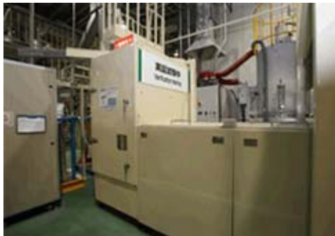
Equipment for removing plastic containing bromine (Equipment for X-ray analysis separation: undergoing testing)
