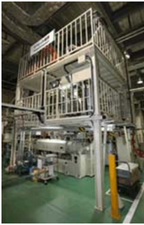
Equipment for removing plastic containing bromine (Equipment for X-ray analysis separation: undergoing testing)
